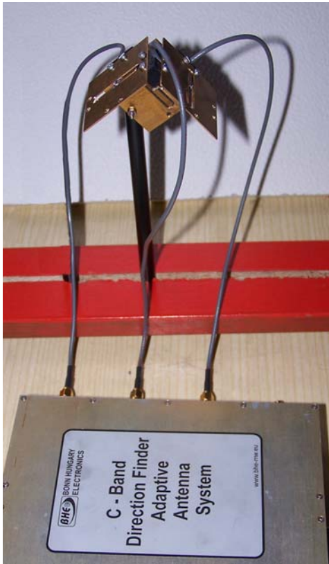
Fig. 7. MIMO antenna with 4 channel receiver
